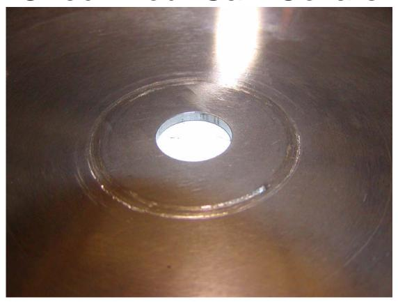
When saw collars get damaged or if the arbor nut is not tightened adequately, the saw blade can be damaged or ruined. Make sure that the collars on your saw are smooth, clean, and properly tightened. Blades that are allowed to spin on the arbor can also ruin your saw's arbor.
