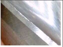
Dull cutting edge at 50X taken out of service before extra damage occurs.
