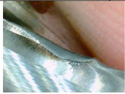
Dull cutting edge on a tool that has been extremely over run.
